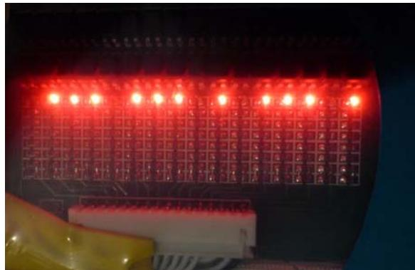
When the pack is being charged and nearly full, the LEDs on the BMS will light up one by one. They're being balanced.
